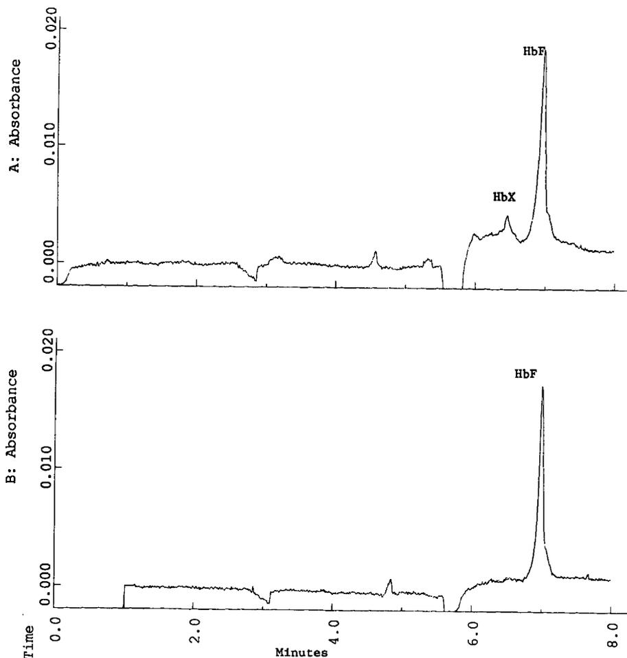
Fig. 4. Separation of hemoglobin F (Hb F) in the sample: (top) in presence, and (bottom) in absence, of an added 100 mg/l of Hb S in the separation buffer (H: new peak). The separation buffer was arginine 2.8 g and Tris 2.4 g dissolved in 100 ml water and the pH was adjusted to 8.5.
