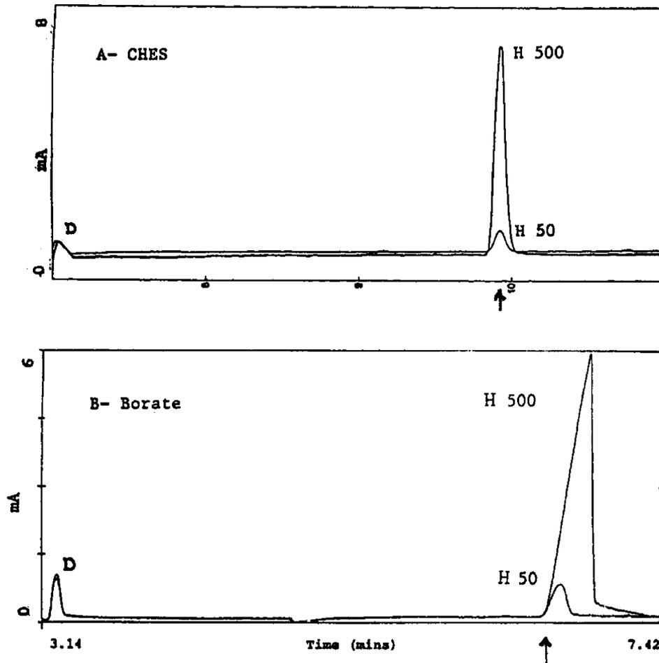
Fig. 1. Effect of both sample concentration and buffer type on migration time for hippuric acid (H): (A) symmetrical peak shape with separation buffer CHES 150 mmol/l, pH 9.0, 214 nm; hippuric acid 500 (top peak) and 50(lower peak) mg/l, and (B) distorted peak shape using separation buffer borate 150 mmol/l, pH 9.0, 214 nm; hippuric acid 500 (top peak) and 50(lower peak) mg/l (D: DMSO; arrow indicates common or constant migration time).
